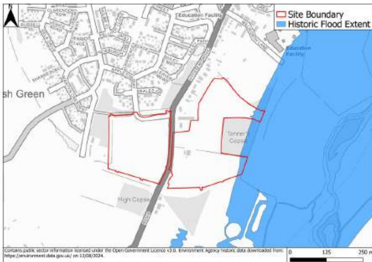
Figure 14 – Historic Flood Extents
