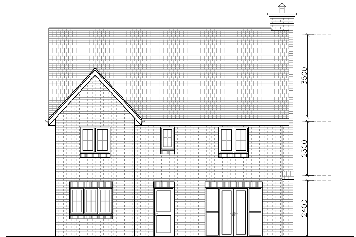
EXISTING REAR SIDE ELEVATION 1:100
