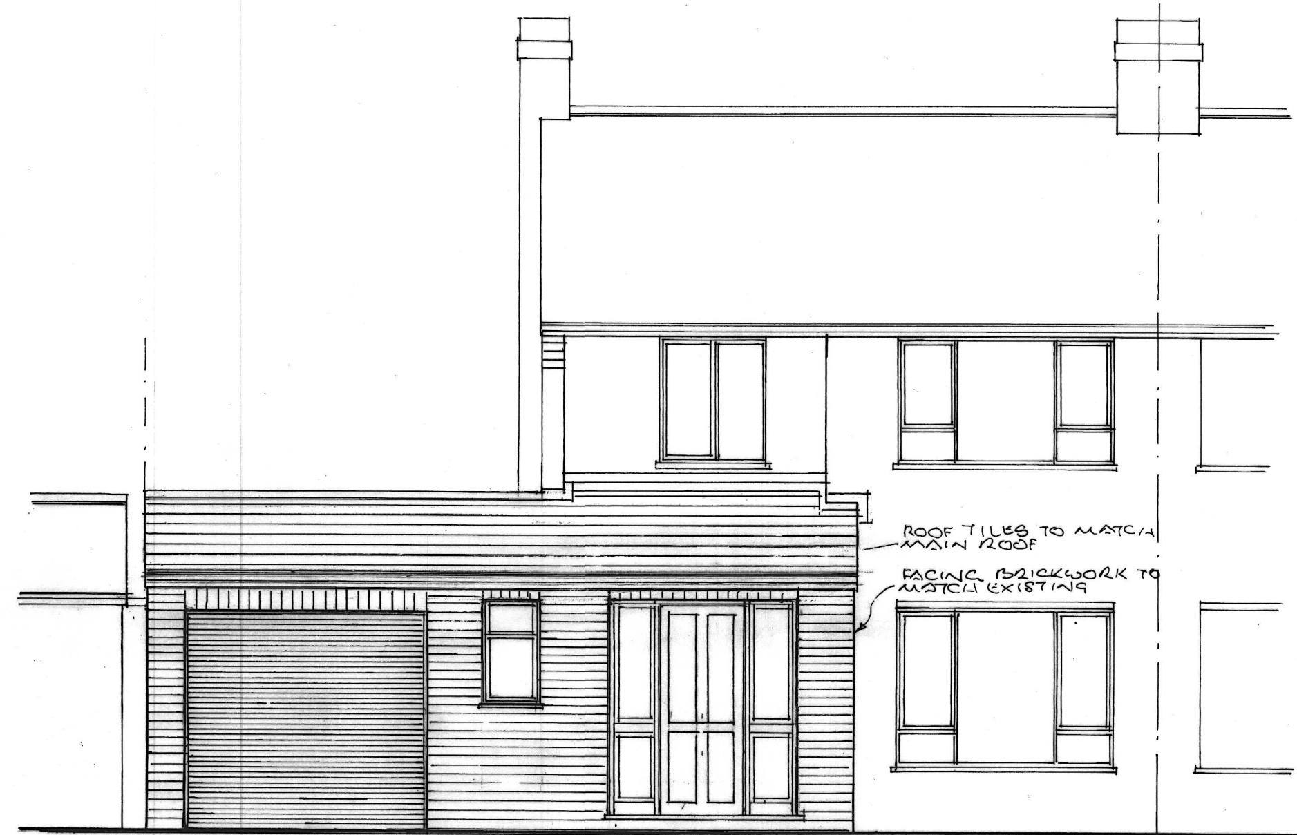
FRONT (NORTH) ELEVATION
