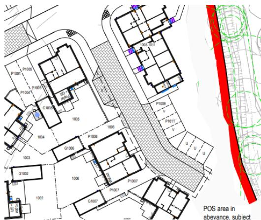
Summary: Risk of junction pull out type collisions as a result of vehicles reversing out onto the highway as turning facilities have not been provided.
