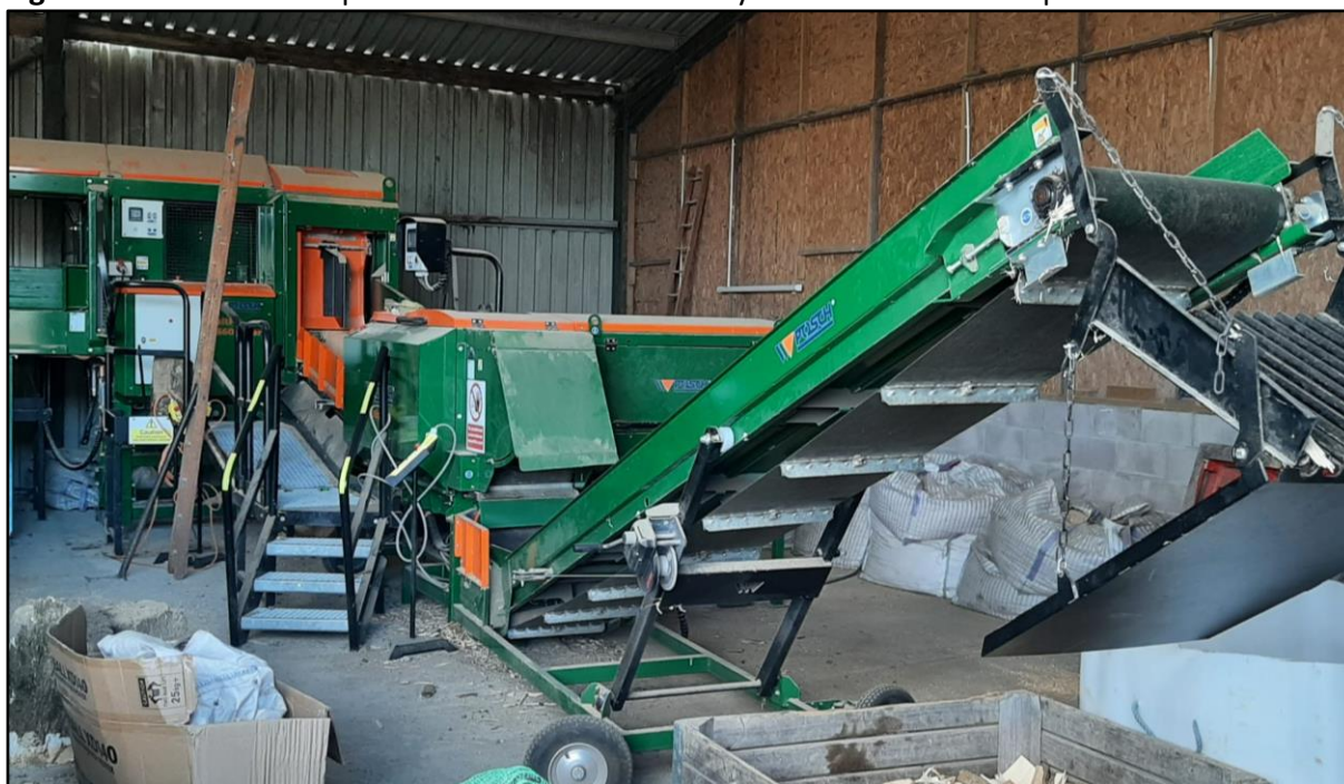
Figure 2: Part of Posch SpaltFix K-700 Vario stationary automatic saw and splitter
