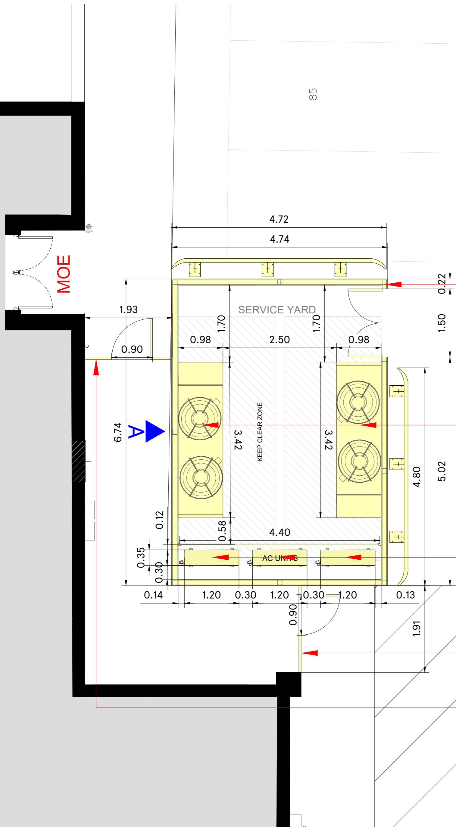
Proposed new 2.4m high hit and miss timber fence enclosure and access gate with Armco barrier on two side to be installed
