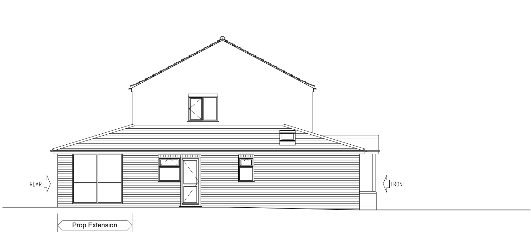
SIDE ELEVATION As Proposed Scale 1:100
