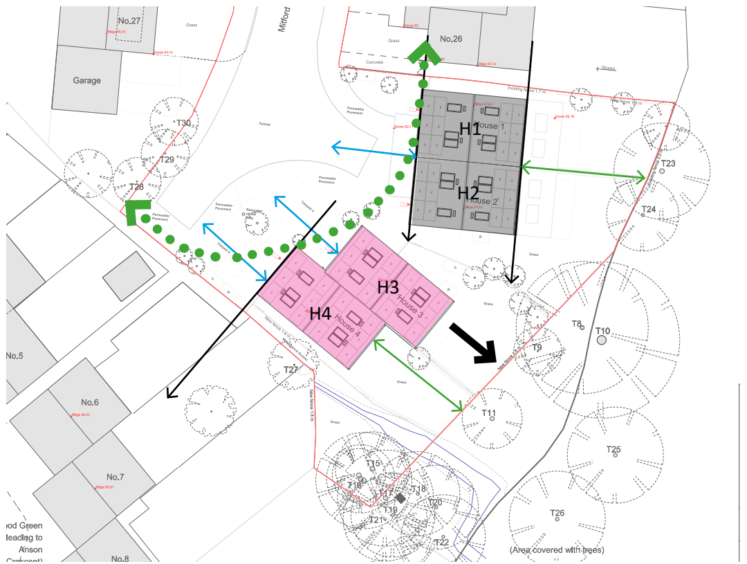
4. Massing adjusted, pushing House 3 backwards to allow for garage access of House 2 and visually, create a harmonious end of street massing (in dotted green).
