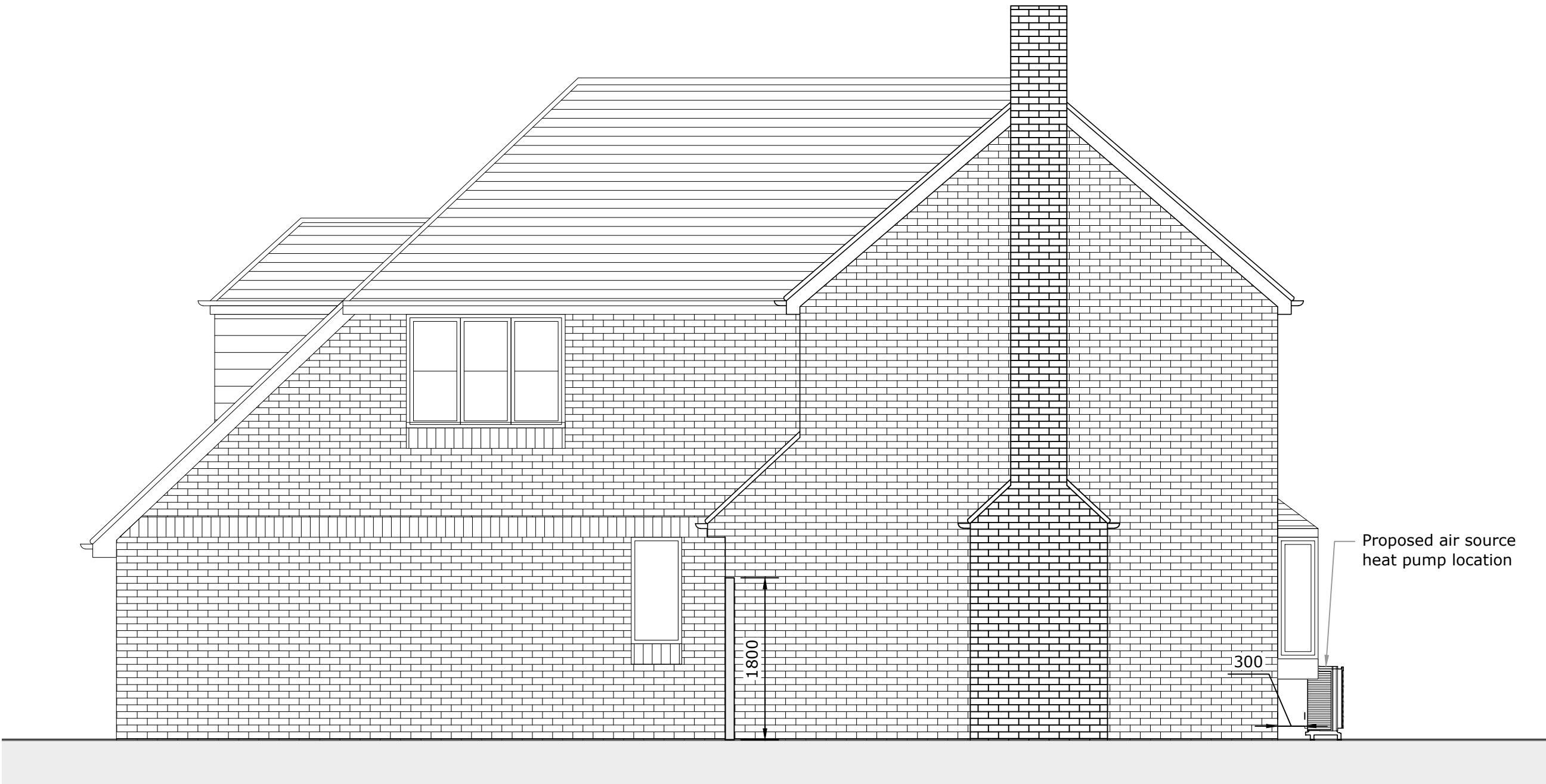
side elevation (east facing) as proposed 1:50
