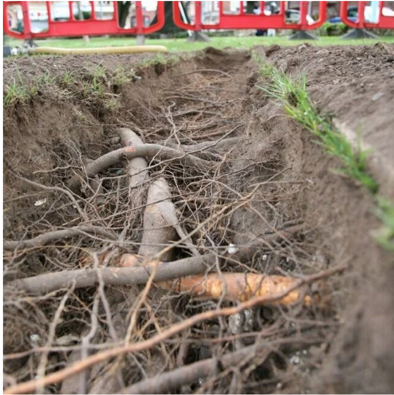
Photo of a trench excavated with an Air Spade exposing the rooting structure.
