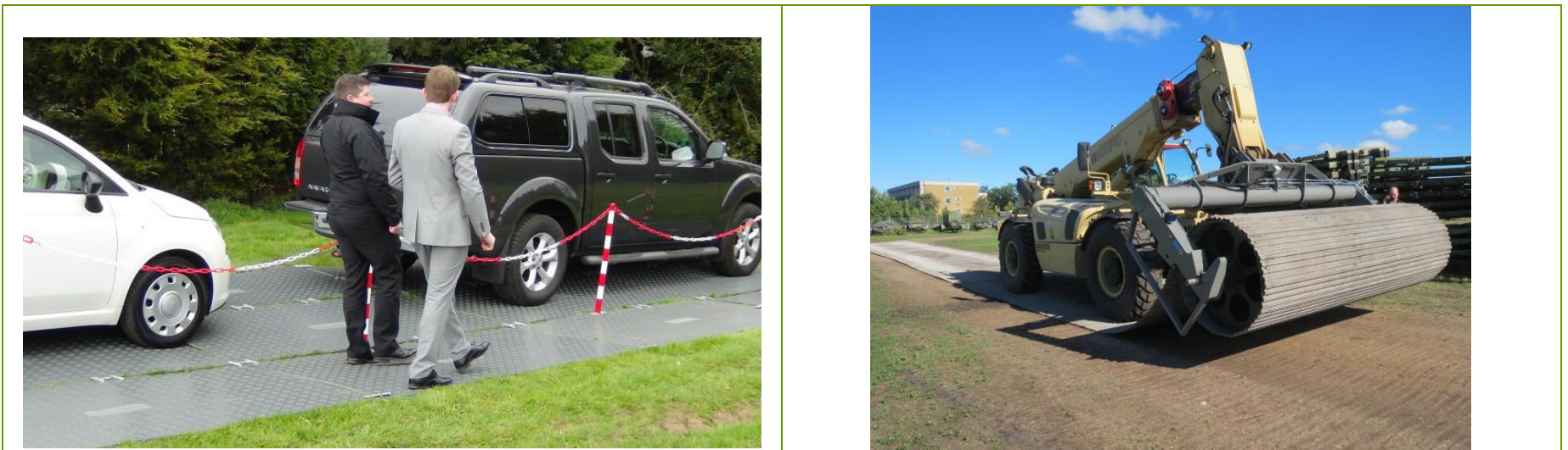
Fig.4: Examples of track board ground protection system – grade will depend on loading to which it will be subject.
