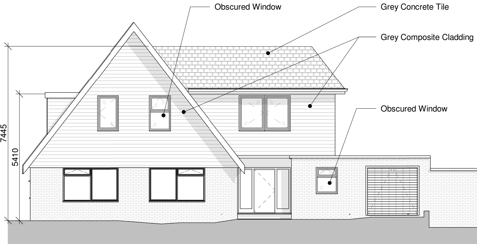
4 Principal Elevation (North) 1 : 100
