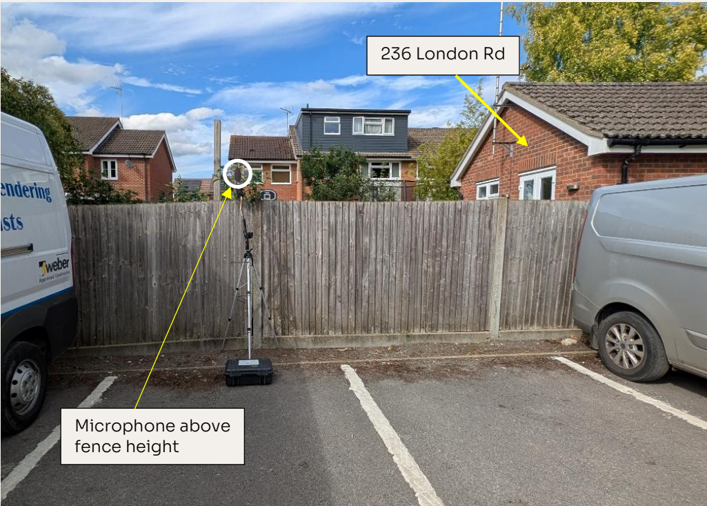
Figure 6 Photo of previous fence adjacent to neighbour, and survey measurement location
