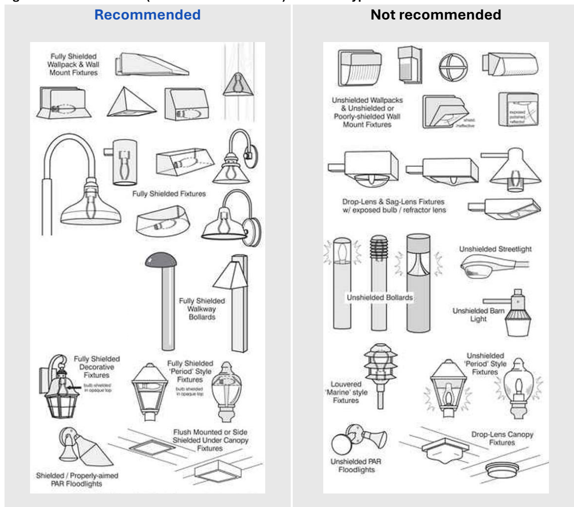
Figure 7. Recommended (and not recommended) luminaire types
