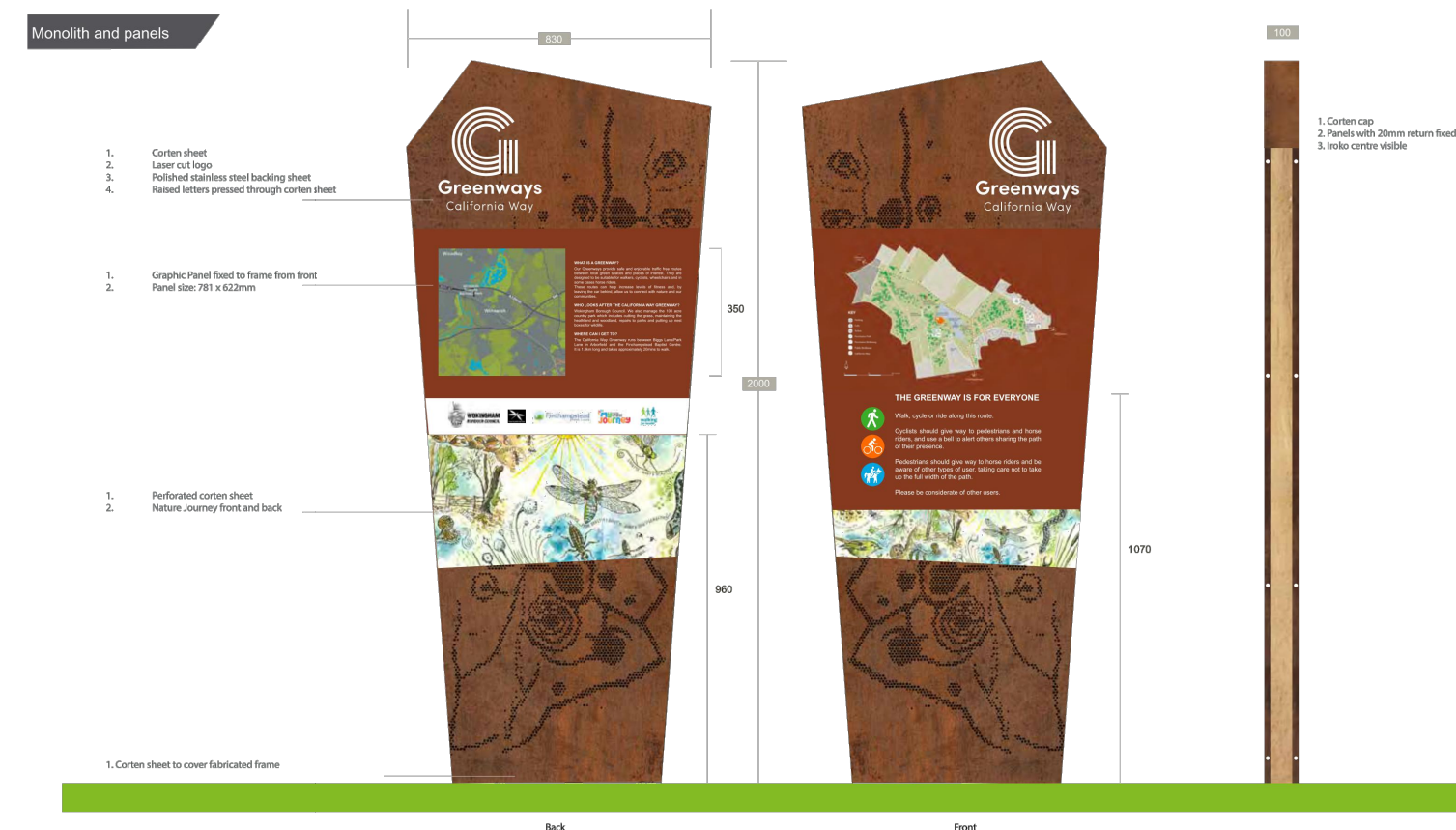
28 TYPE B.2 WAYFINDING SIGN ELEVATION SCALE - 1:20 @ A1 & 1:40 @ A3
