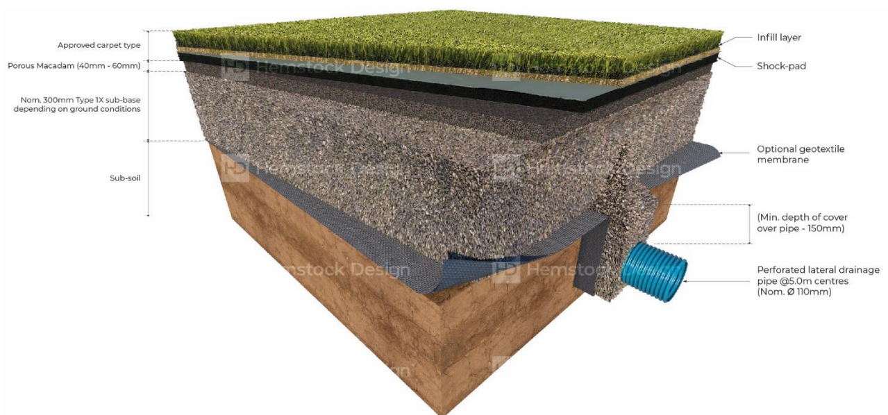
Fig. 6 - Illustrative profile of the new MUGA ATP, with sand infill needle-punch carpet over a porous bitmac layer (possibly with shock pad), with drainage layer aiding attenuation of peak flows
