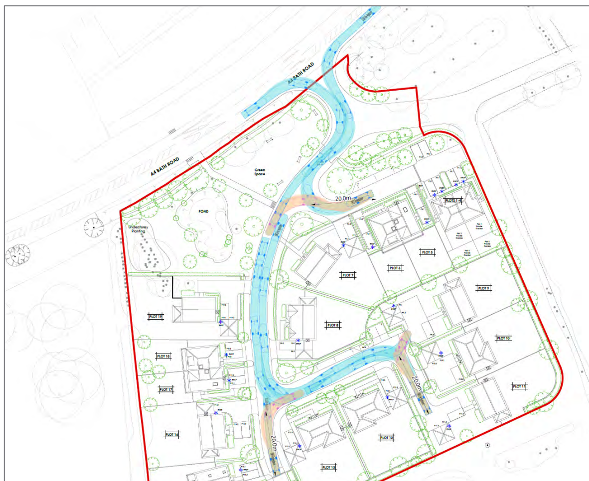
Image 3.1: Revised Fire Appliance Swept Path Analysis – DB32 Vehicle
