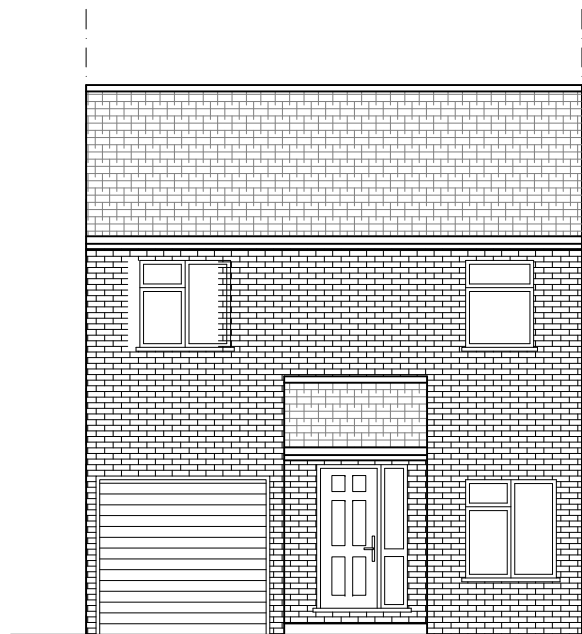
Existing Front Elevation
