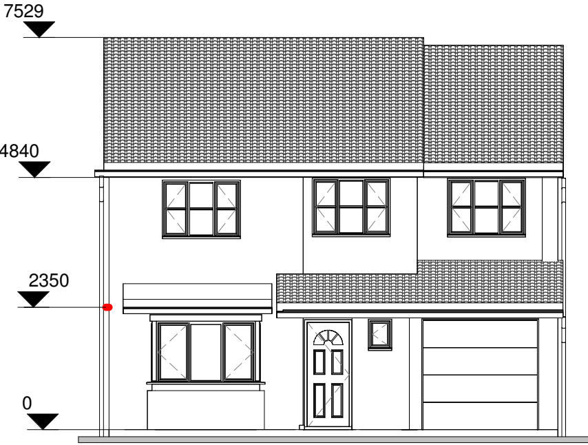
Existing Front Elevation 1 : 100
