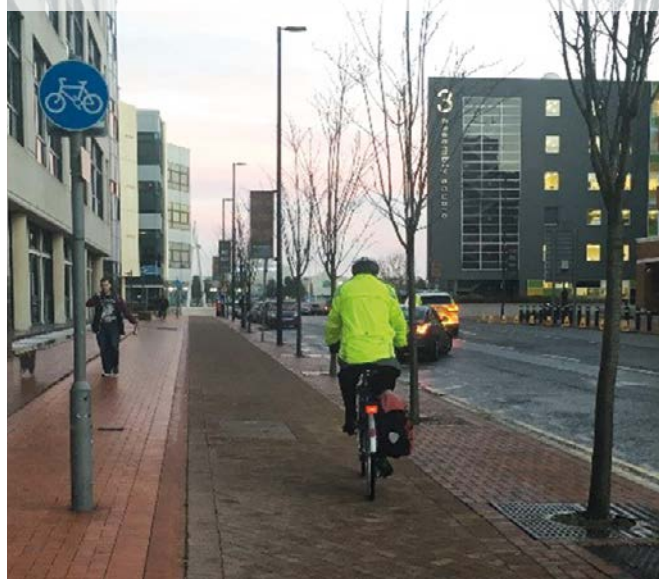
Figure 6.14: Cycle track with sign to TSRGD diagram 955
