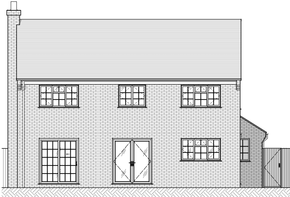
Existing Elevation - South
