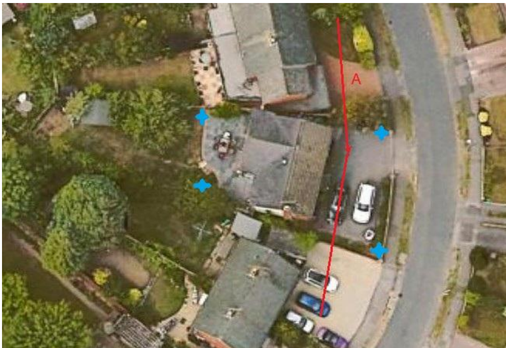
Figure 1. Surveyors and cameras (blue stars). Flightpaths (red line)
