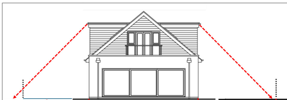
Figure 6 Vertical 45-degree angle test
