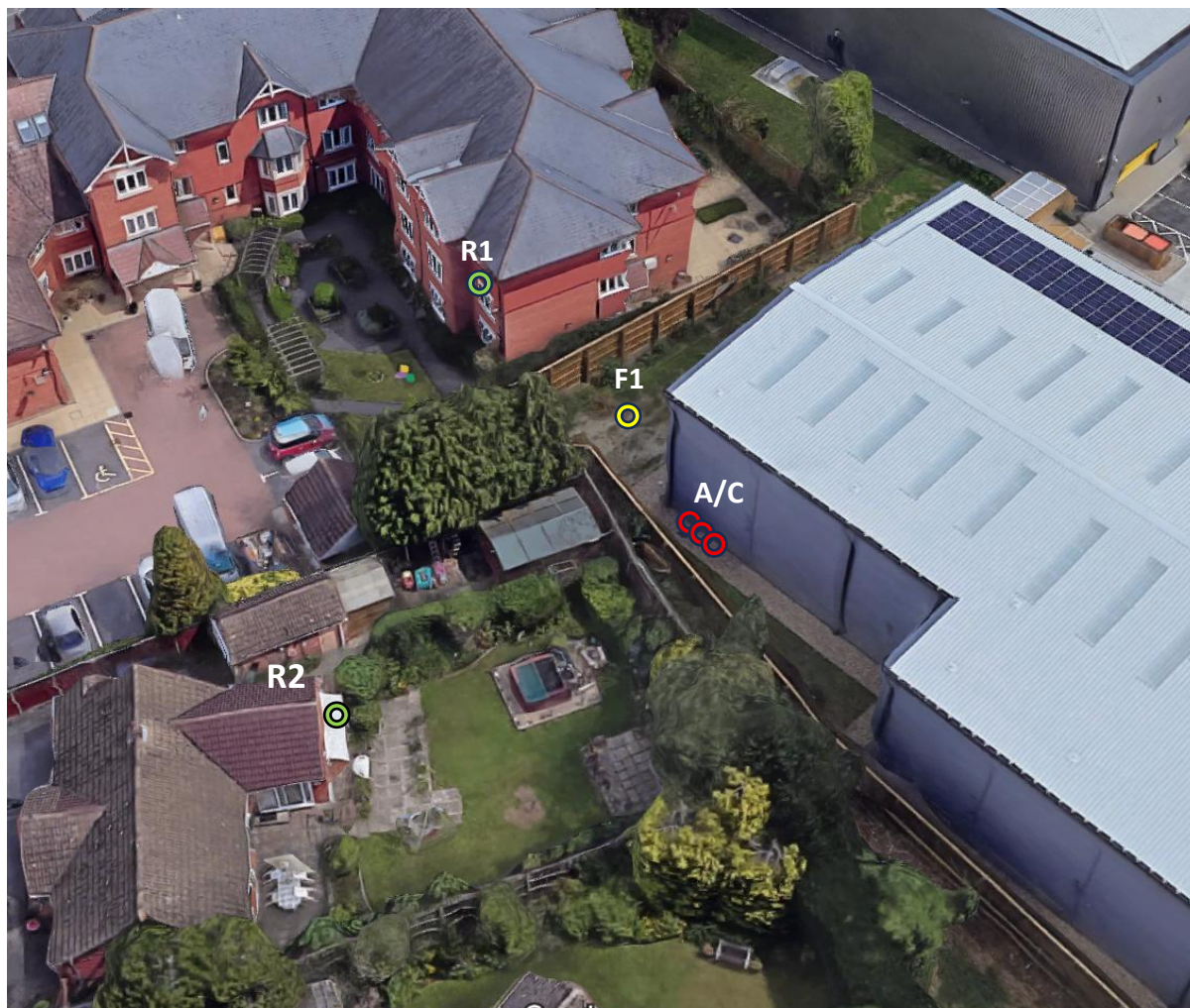
Figure 3.1 Aerial view of site with survey location (F1), nearest receptor façades (R1, R2), and proposed A/C location (red)
