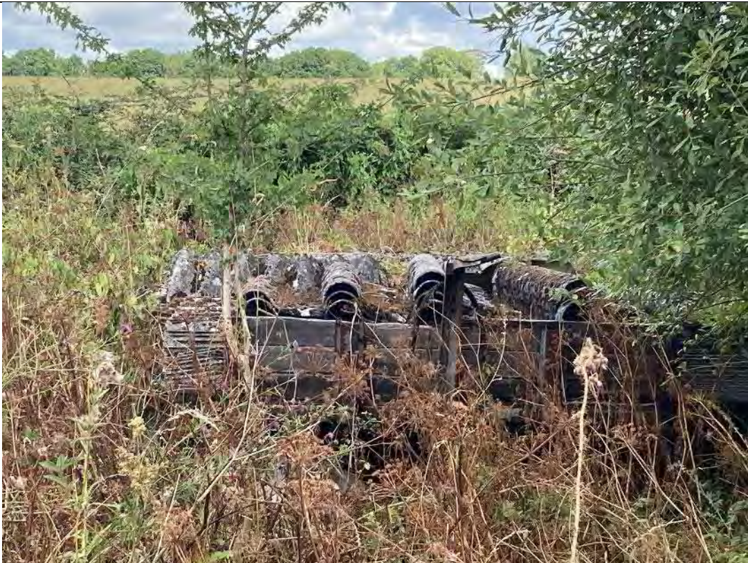
Photograph 25 – PACM tiling within a trailer located in the northeast corner of Area 2
