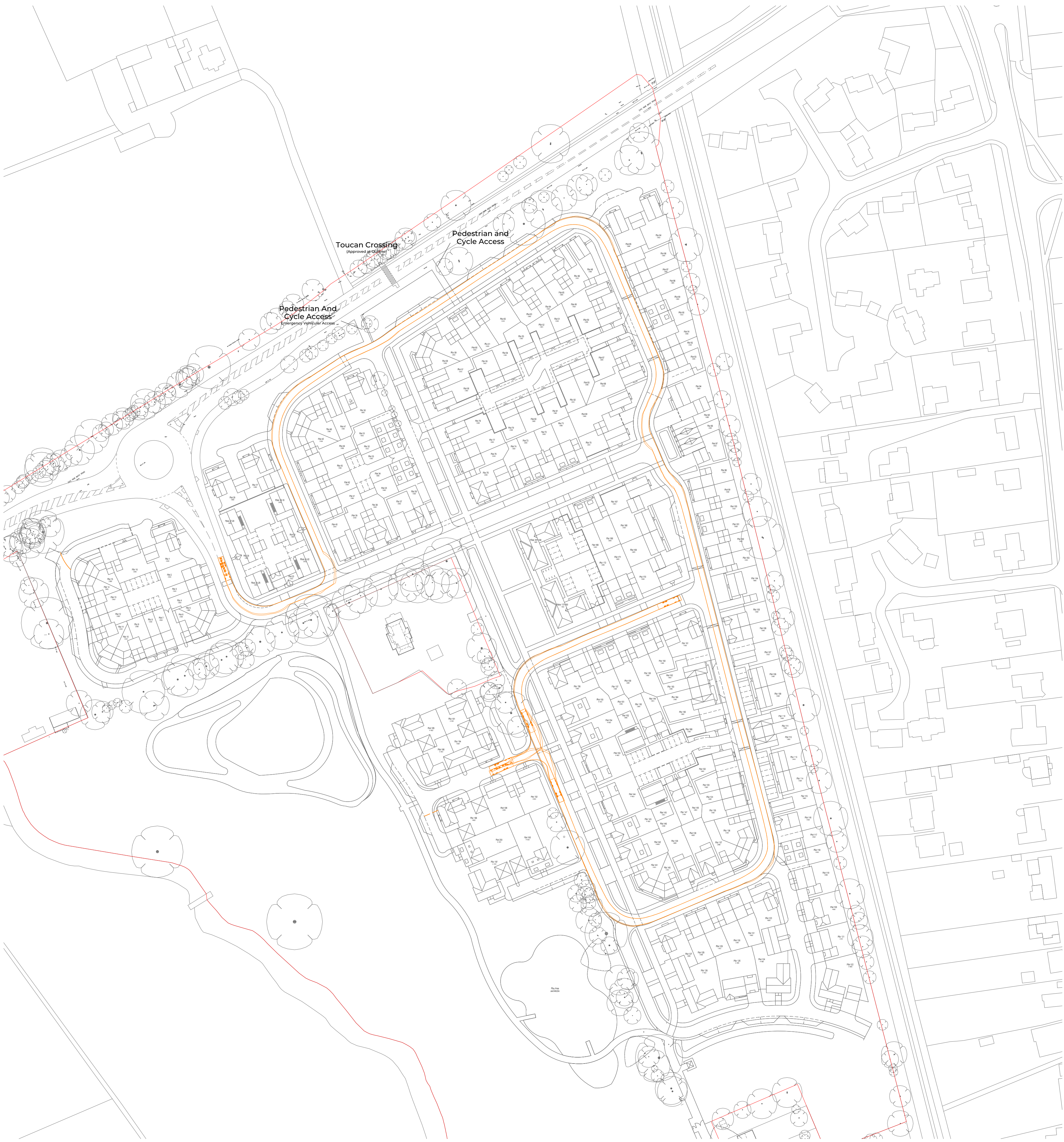
Refuse Vehicle Tracking (With Car Passing) Scale - 1:1000
