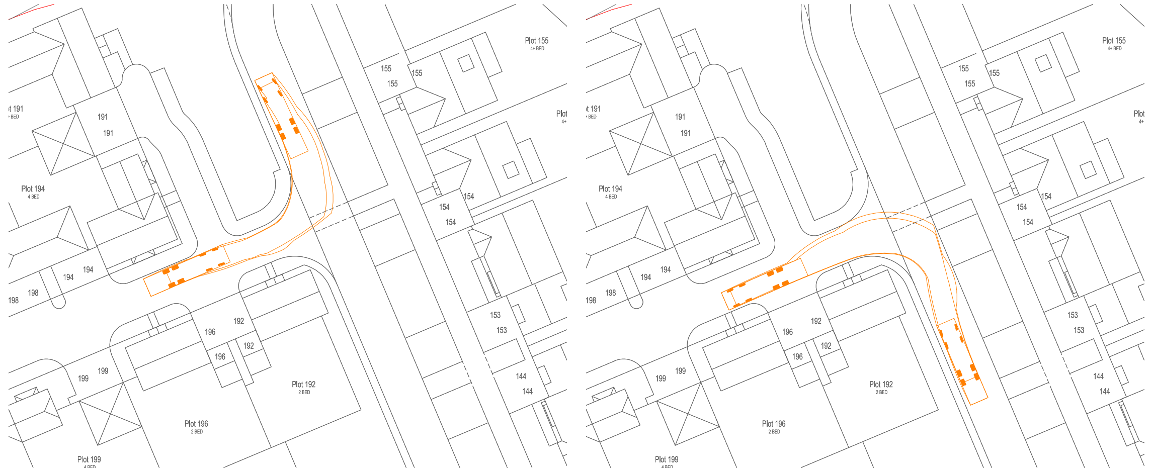
Refuse Access - Key Junction
