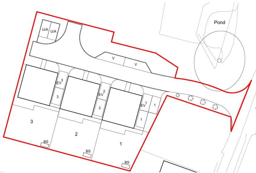
Image 12 – Proposed layout of the dwellings, access and parking (extract from the Proposed Block Plan)
