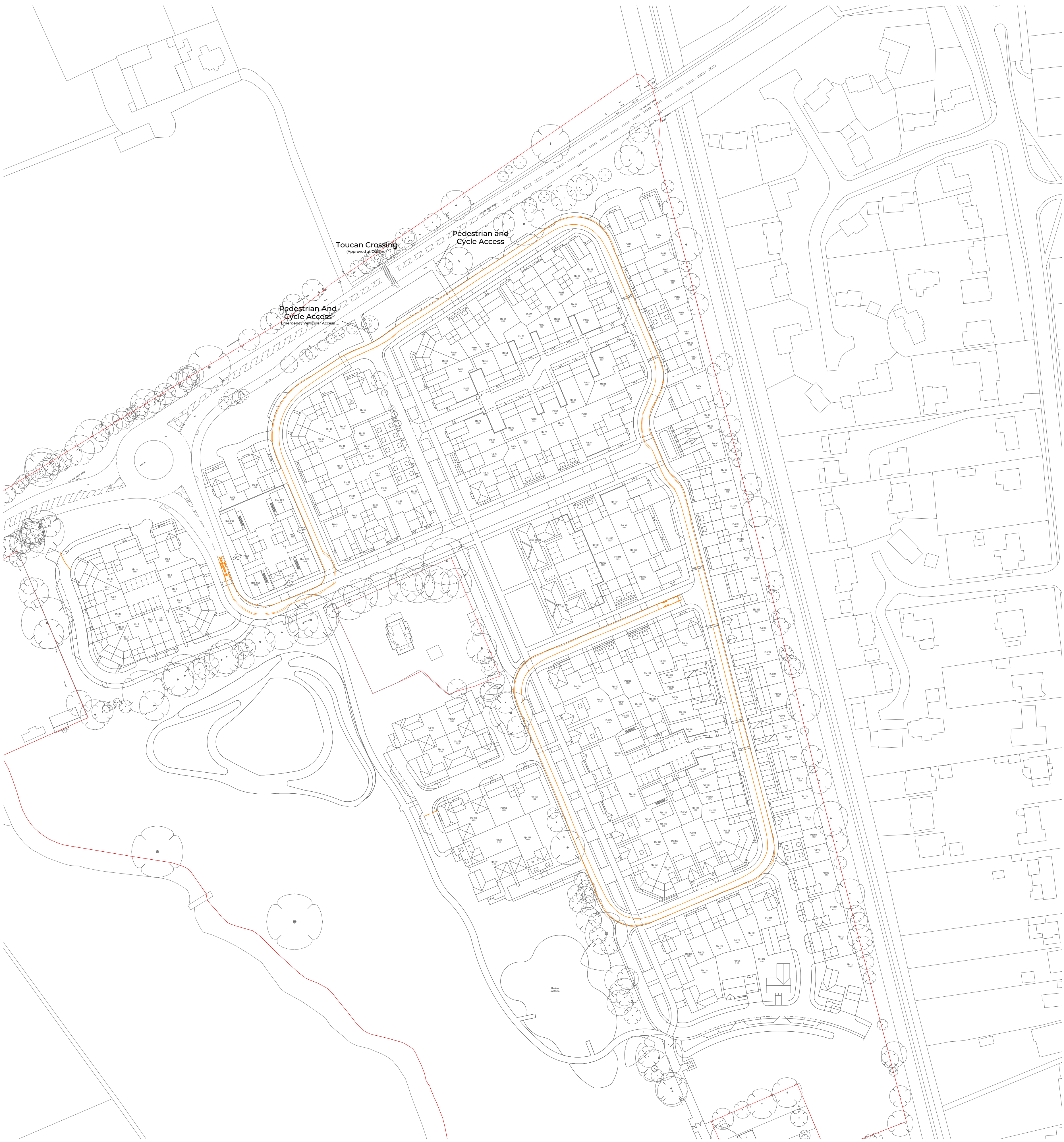
Refuse Vehicle Tracking (With Car Passing) Scale - 1:1000
