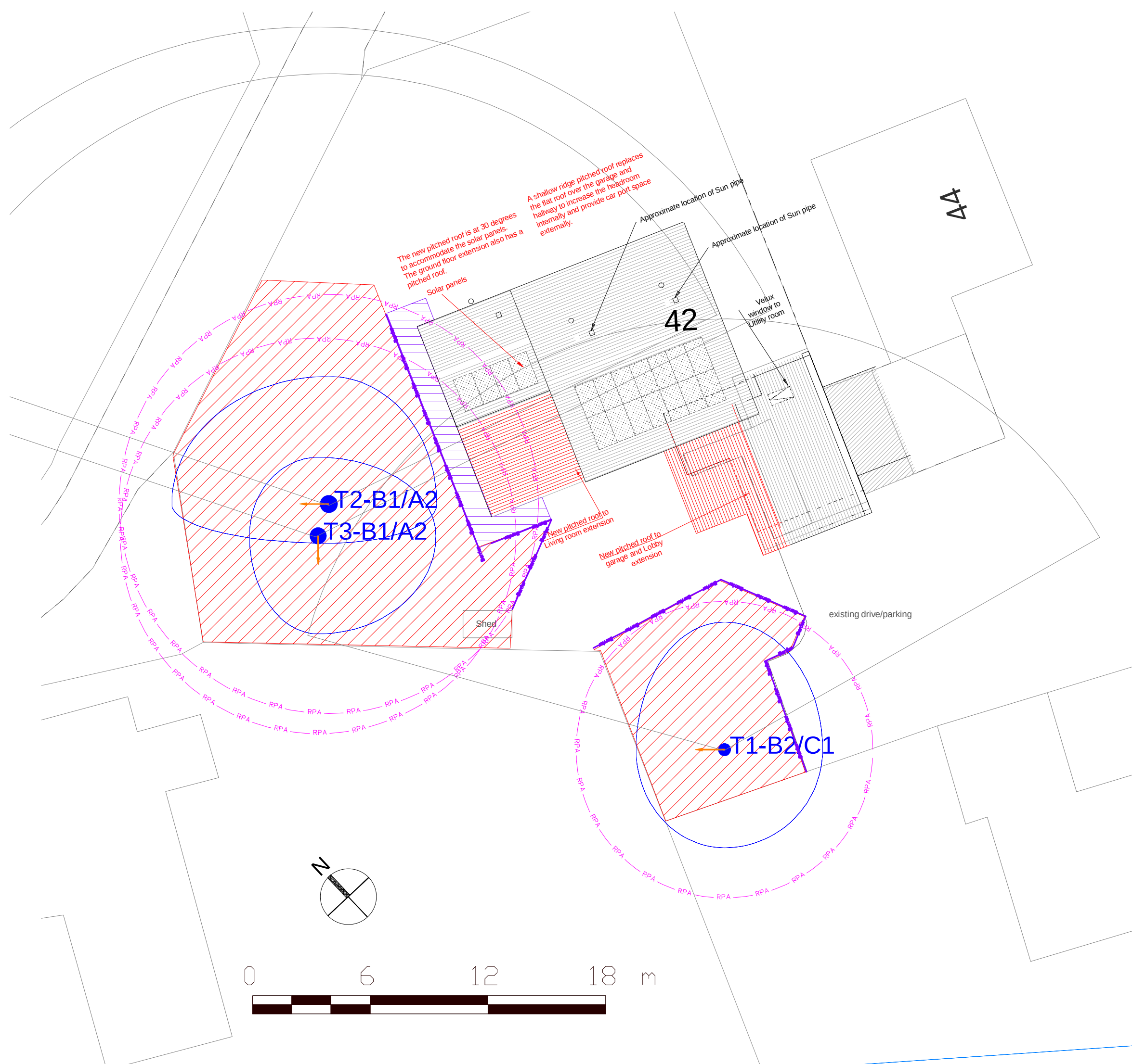
Figure 3 BS 5837 : 2012 - Default Specification for Protective Barrier
