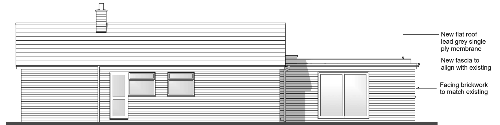
SIDE ELEVATION (facing 10 Woodrow Drive) 1:100
