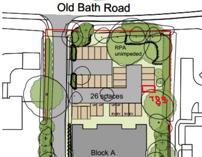
Fig. 1 An incursion into the root protection area of 'B' quality Oak T83 a protected tree from the additional parking bay. No RPA on this drawing to fully assess the impact.
