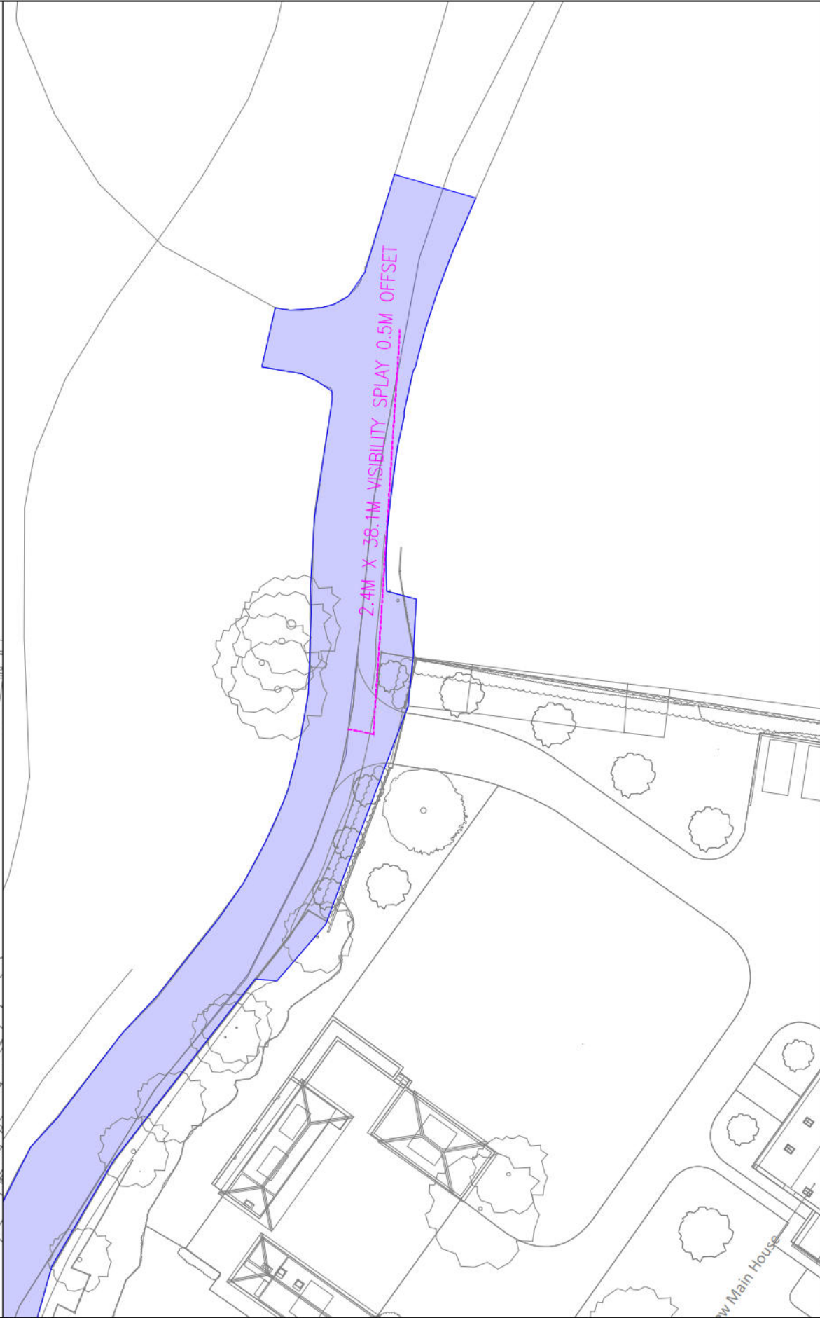
MAXIMUM ACHIEVABLE VISIBILITY NORTH WITH 0.5M OFFSET AND 2.4M Y DISTANCE
