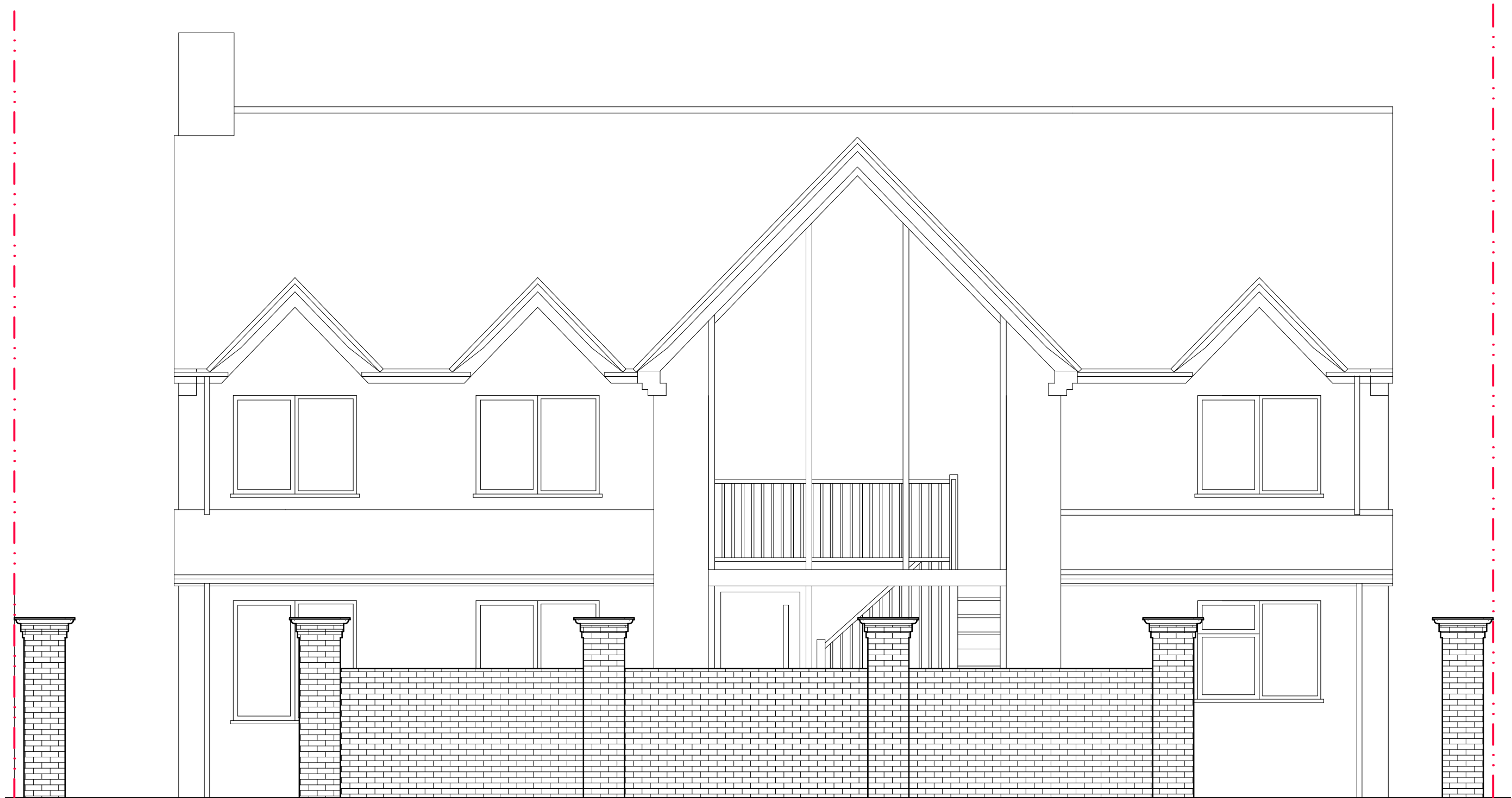
PROPOSED REAR ELEVATION OF BOUNDARY WALL
