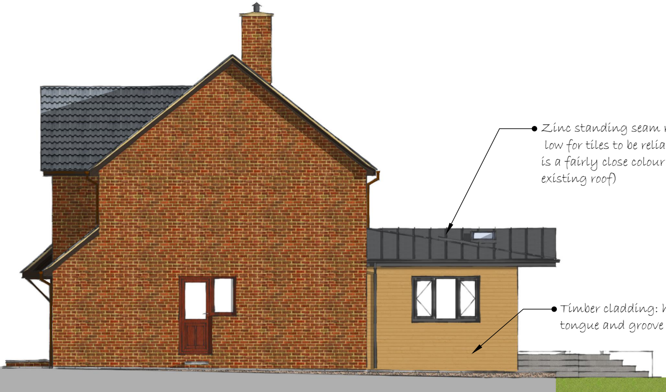
Side Elevation (North)
