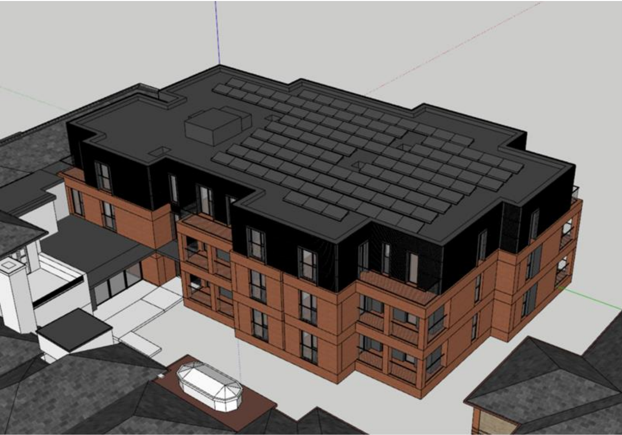
Figure 7. Roof PV Layout.
