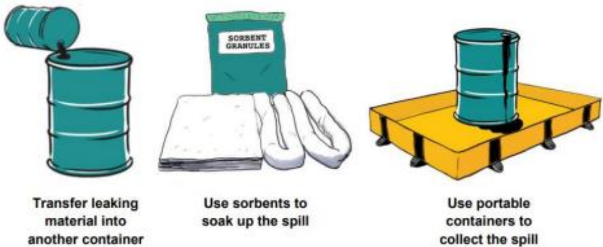
Examples of how to control a spill close to the source
