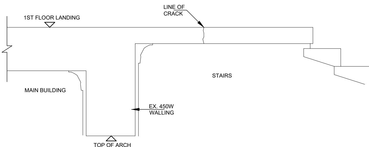
EX. SECTION AT ARCH OPENING - UNDERSIDE
