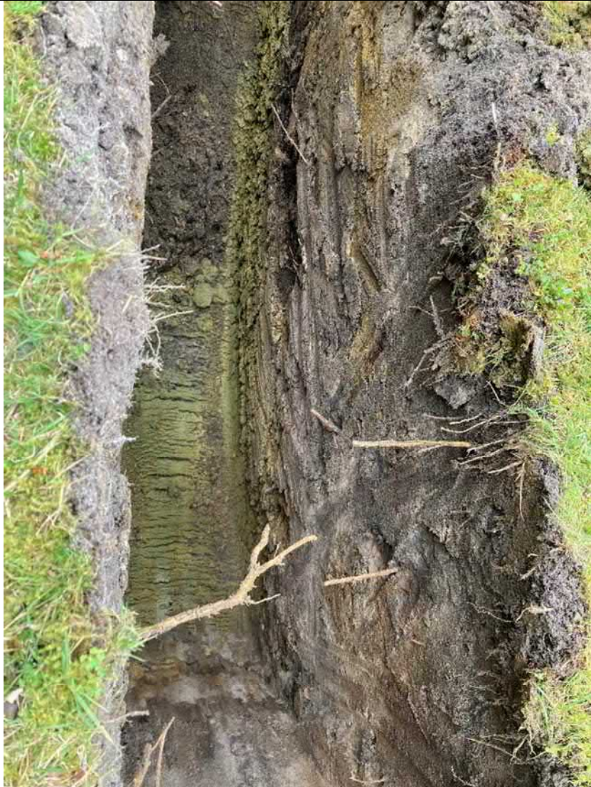
Photograph 4 – SA102 Trial pit, Windlesham Formation at the base.
