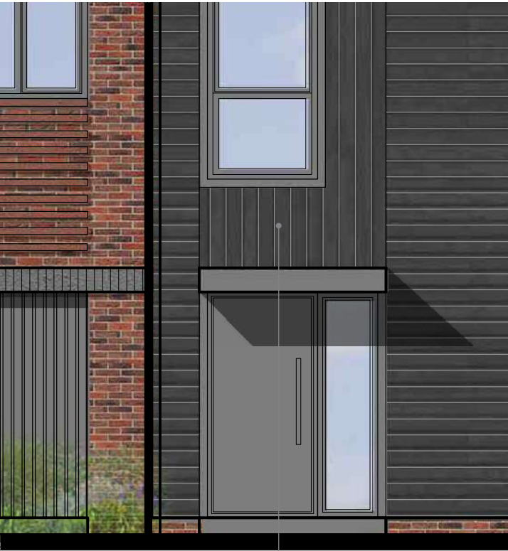
Combination of vertical and horizontal weatherboarding to gable marking core
