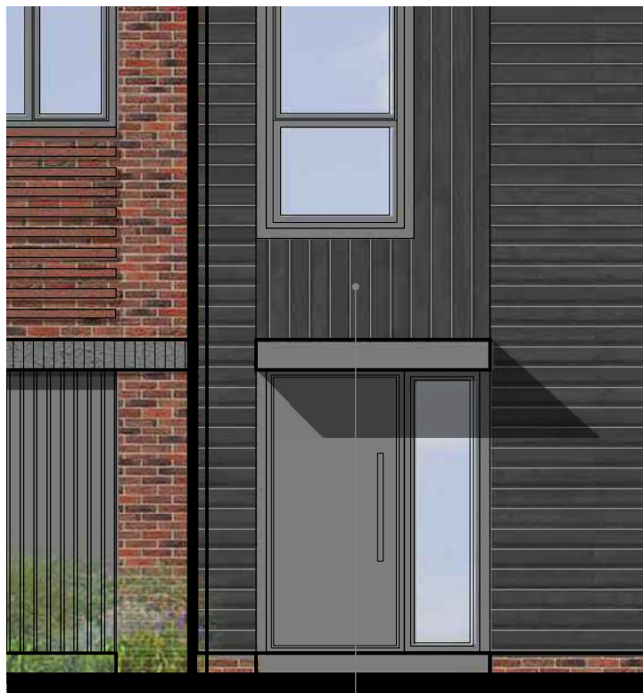
Combination of vertical and horizontal weatherboarding to gable marking core
