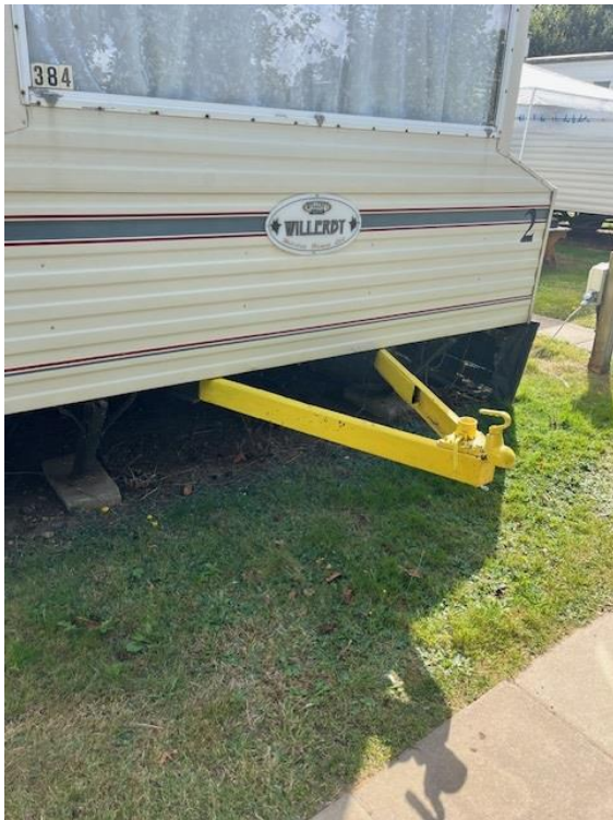
Photo.2 – towing hitch on mobile home
