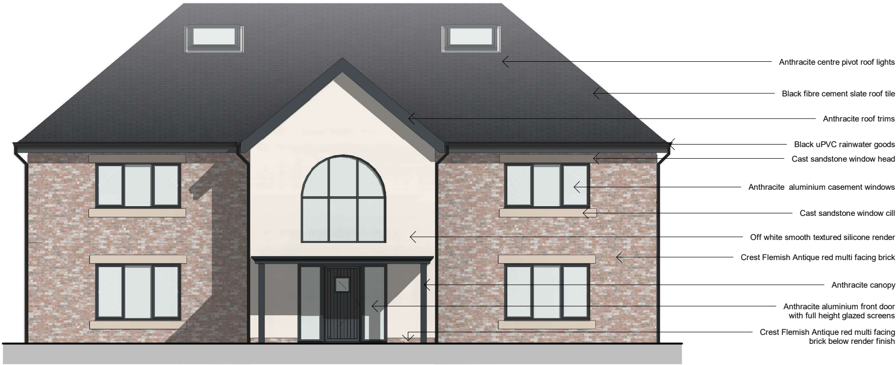
PROPOSED SOUTH ELEVATION 1 : 100
