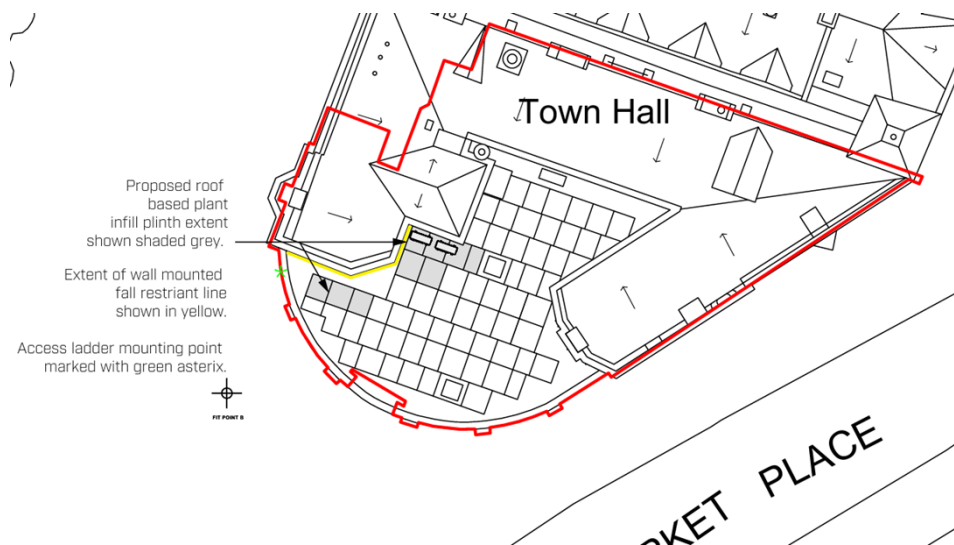
Extract from Drawing No. 1323-Ww-B1-00-DR-A-0010: Proposed Site Layout
