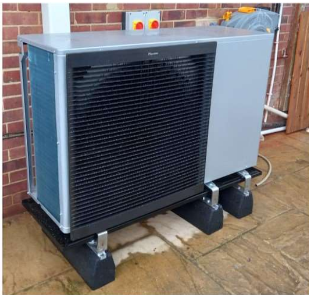
EDLA 9/11/14/16kw Dimensions: Length 1380mm Depth 460mm Height 870mm Add 150mm for feet Drip tray option add another 100mm
