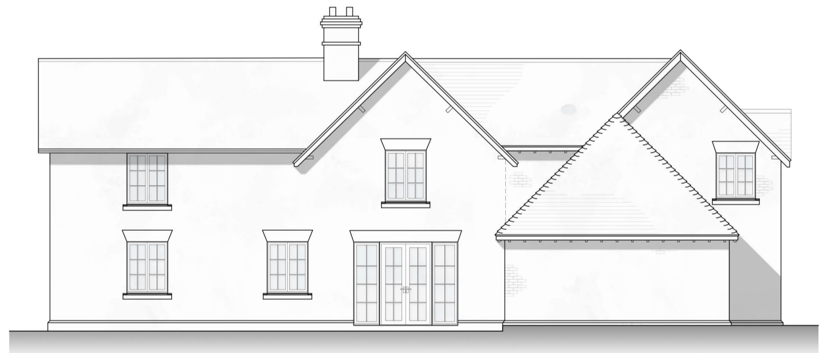
REAR ELEVATION (south east facing) Scale 1:100 @ A1
