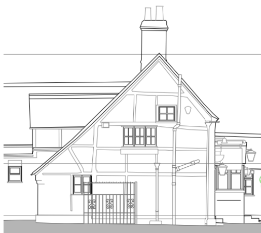
Both drawing PL.020 Rev. P1: Existing North Elevation (image to left) and drawing PL.023 Rev. P3: Proposed North Elevation (image to right) both include along with the historic timber framing of the north gabled end wall of the Swan, the faux painted on timber elements, which were omitted when the walling was repainted
