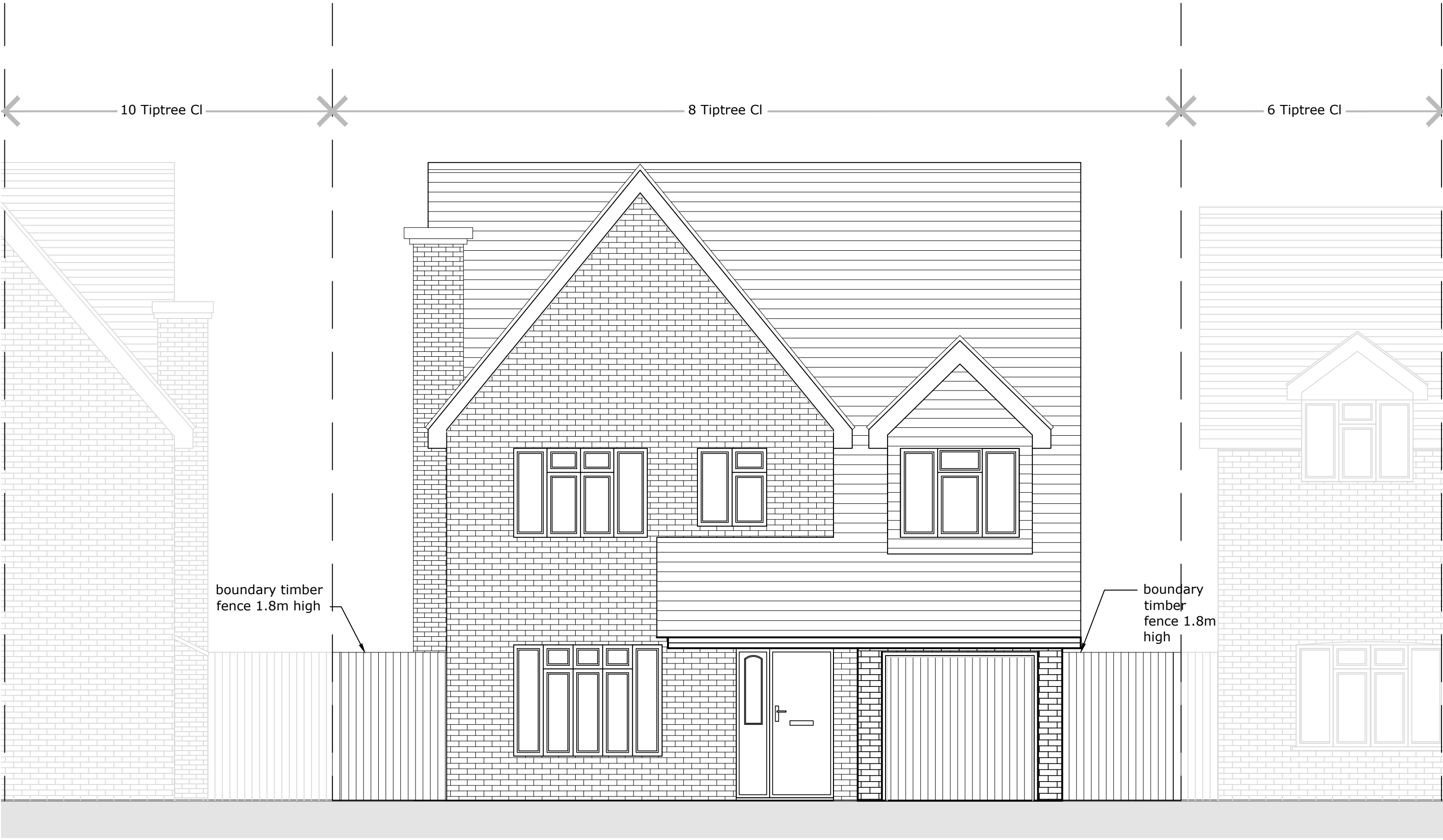
front elevation (west facing) as proposed 1:50
