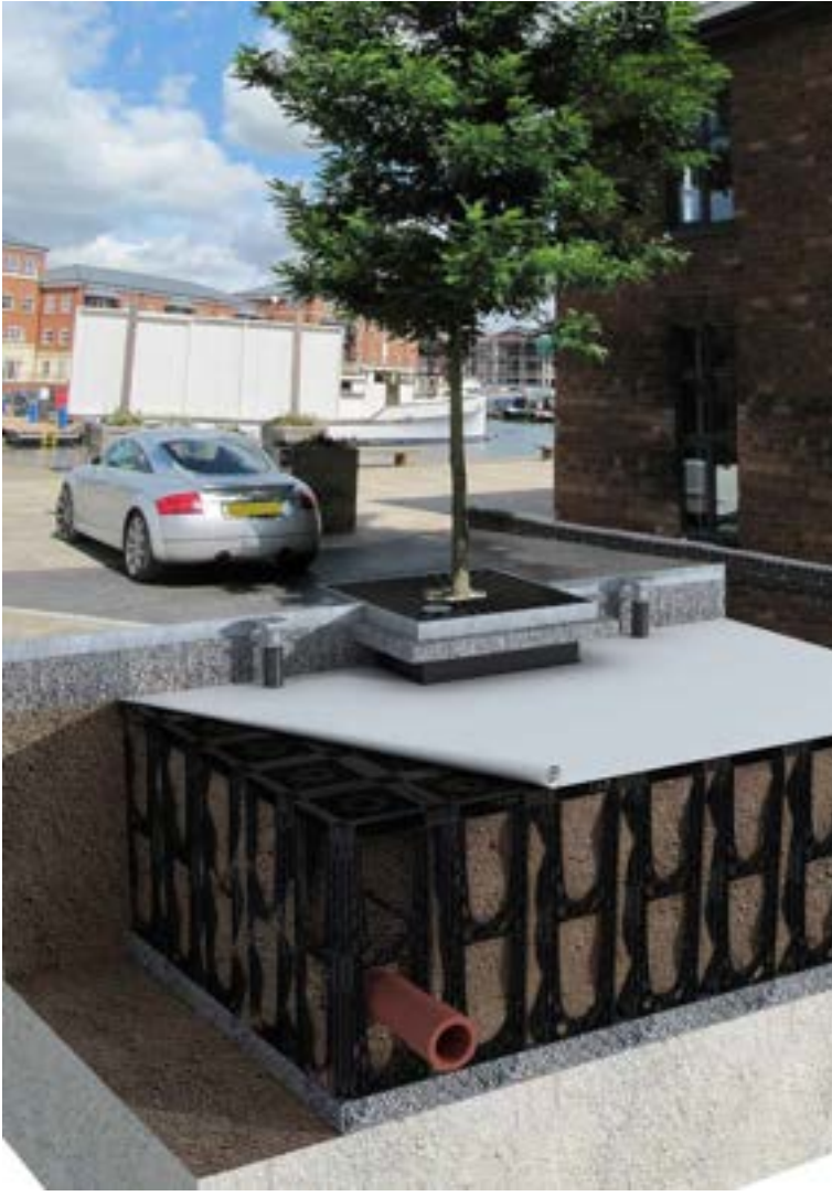
GreenBlue Urban RootSpace soil cells
