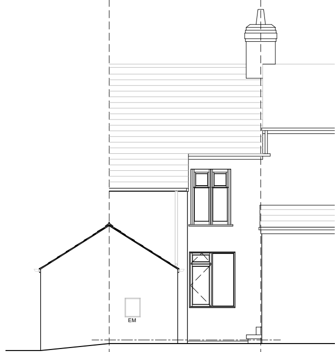
REAR ELEVATION As Existing Scale 1:100
