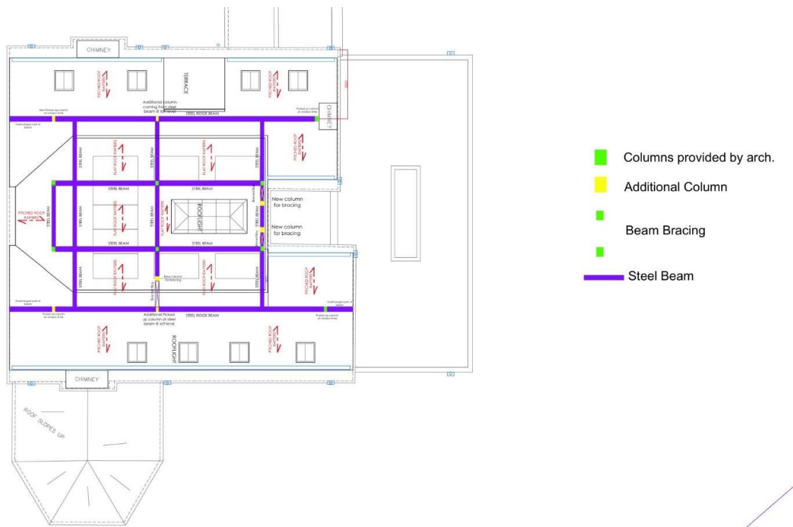
Photo 4a and 4b – Main House Plan – New Roof - Indicative /concept structural member framing at loft and roof level.
